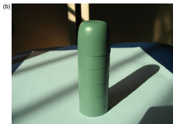
Fig. 3. Photos of (a) the green anode substrate by dip coating technique compared with the sintered one and (b) the anode substrate stack. (For interpretation of the references to color in this figure legend, the reader is referred to the web version of the article.)
